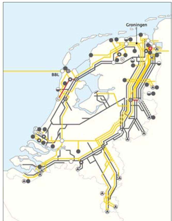
Overzicht gastransportnetwerk © Gas Transport Services
