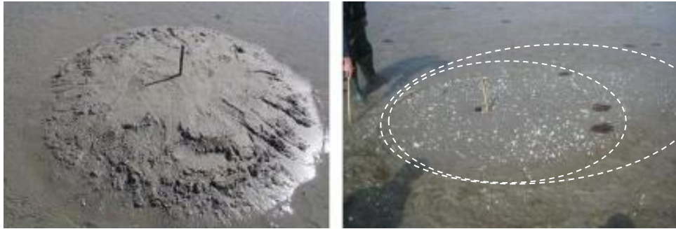
Figure 2 Mini sand nourishment after building (T0, left photo) and after a 48h period (right photo). The inner circle denotes the original position of the mini sand nourishment, the outer circle the position of the sediment after 48h.
