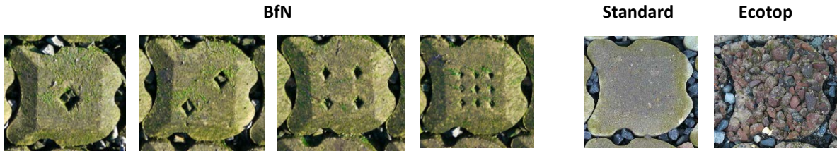
Fig. 6. Specimens of: the four different types of BfN blocks; a standard hydroblock; and a hydroblock with lavastone ecotop, a few weeks after placement at Sint-Annaland.
