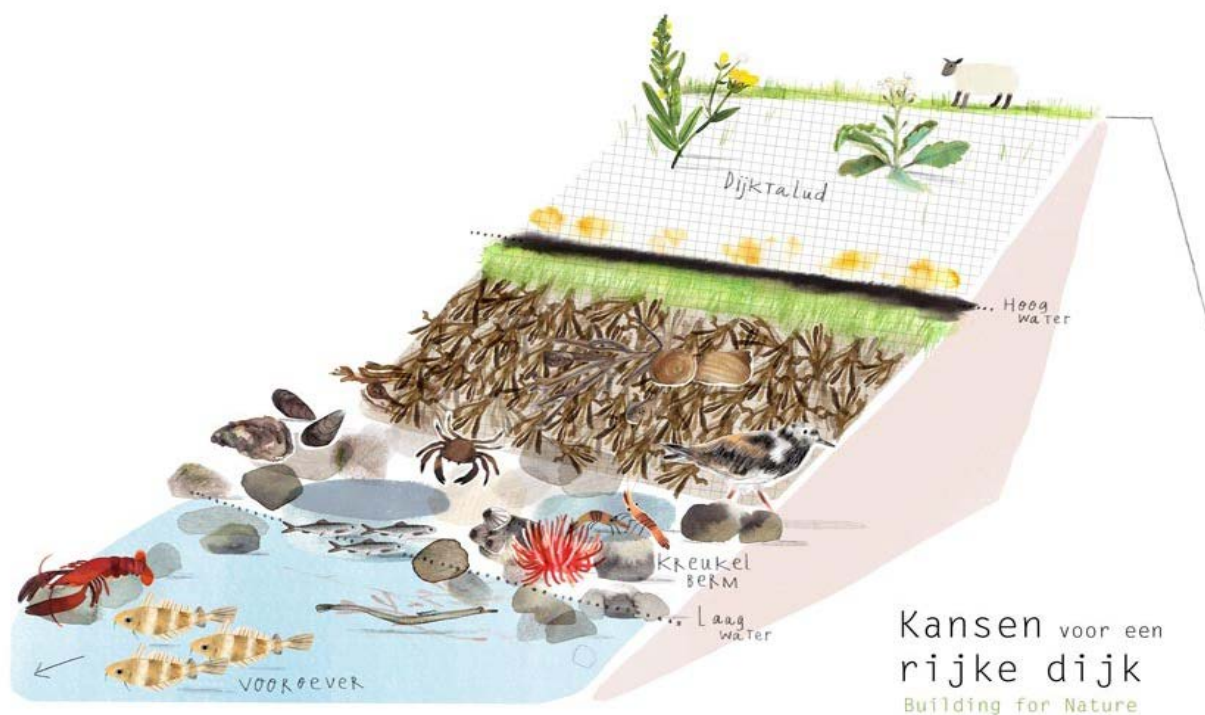
Fig. 1. An artist impression of a 'rich revetment' with a high biodiversity on the revetment, the riprap at the toe and in the foreshore (illustrator: Ruth Hengeveld).
