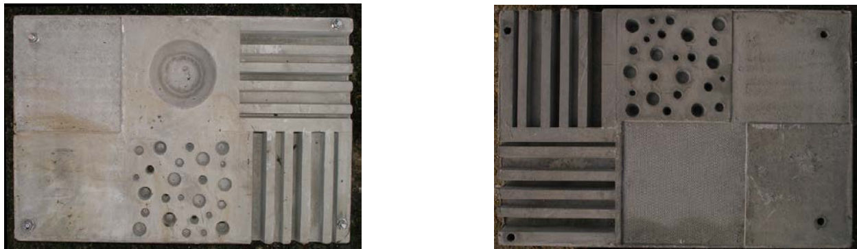
Figure A5-1. Left: a concrete plate for horizontal installation. Right: a concrete plate for vertical installation. The horizontal plates have one smooth surface, one surface is roughened at a mm scale and four surfaces are roughened at a cm - dm scale. The vertical plates have one smooth surface, two surfaces roughened at a mm scale and three surfaces roughened at a cm - dm scale. Both horizontal and vertical plates have one surface with pits with varying widths and two surfaces with crevices of varying widths. Crevices at the vertical plates are horizontally and vertically orientated.
