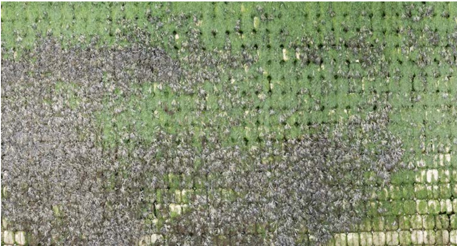
Section 12: Hillblocks. Left part:porous; right part: standard. April 2016
