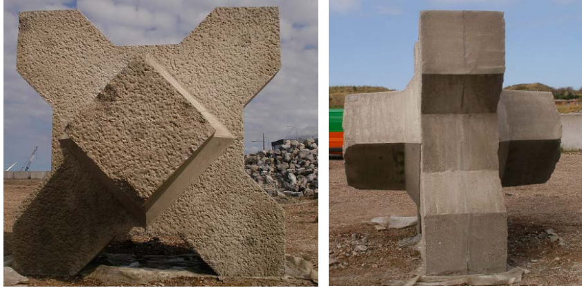
Figure A5-4. The eco-X-block with one roughened side and one side with a smooth surface.
