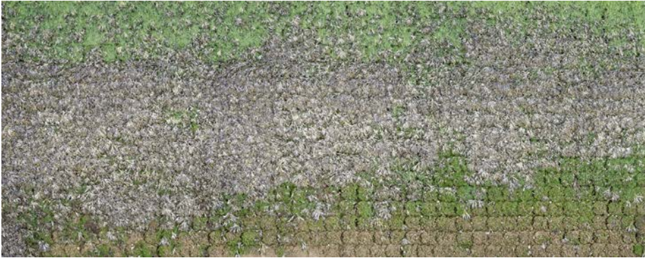
Section 12: Hillblocks. Left part:porous; right part: standard. April 2016
