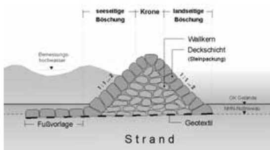
Standard cross-section of a breakwater, StAUN (2009)
