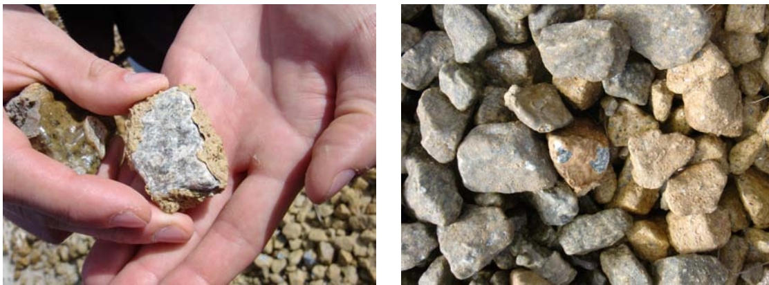
Figure 5-1: Example for a quality defect caused by residual moisture on the granular material during the mixing process (Photos: IMS)
