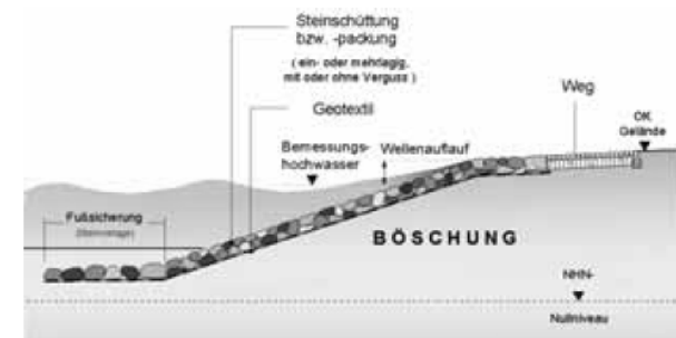
Standard design of a revetment, StAUN (2009)
