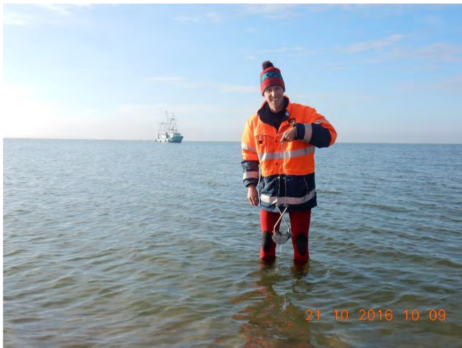
Figure 0-3 Taking sediment samples with a Van Veen Grabber. In the background is the ship at the location of the hydrodynamic measurements
