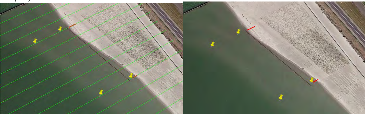
Figuur 2 Location measured depth rows and sediment sampling locations (red line are the sampling locations taken with a Van Veen grabber, yellow markers are the locations of sediment core samples with piston sampler)
