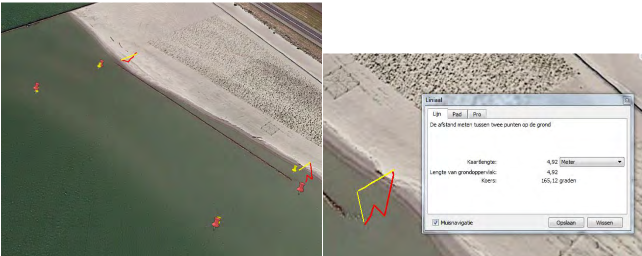
Figuur 3 Left: Proposed sampling locations displayed in yellow and the actually sampled locations displayed in red Right: Largest deviation in sampling locations lies within the accuracy of the GPS
