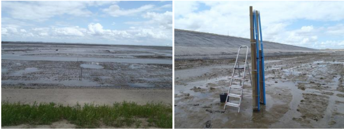
Figure 3.5. Piezometers in tidal area during low tide (left) and nest of 3 piezometers installed at different depths (3, 8 and 12 m bgl)
