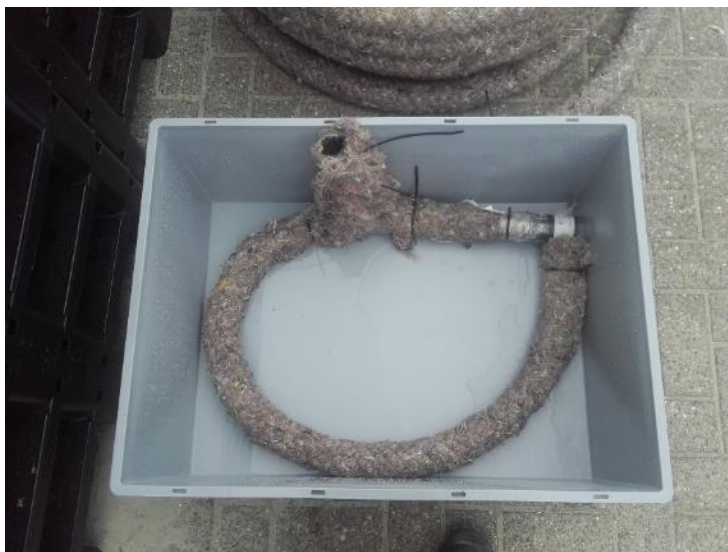
Figure 4.4. Drainage system in mega-marsh organ
