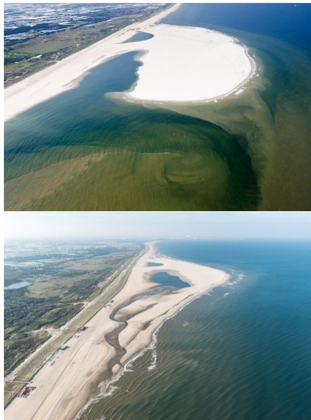
Figure 8: Upper panel: The Delfland Sand Engine shortly after placement (July 2011). Lower panel: The Sand Engine has evolved into an almost symmetrical salient (October 2013). (Source: https://beeldbank.rws.nl , Rijkswaterstaat / Joop van Houdt)
