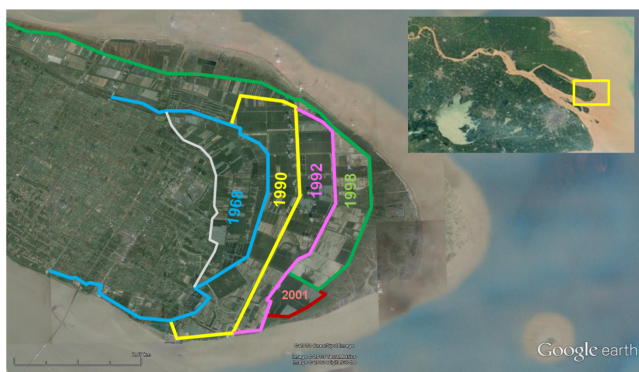
Figure 17: Consecutive reclamations of accreted marsh on East Chongming Island, Yangtze Estuary, China.
