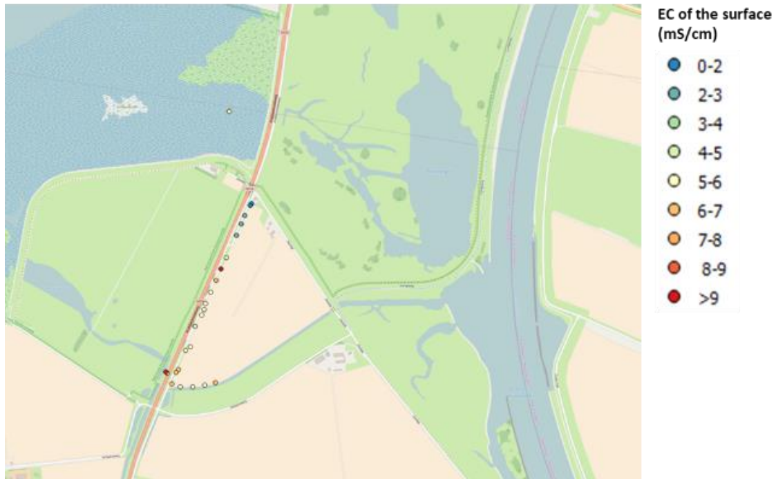
Figure 35. Results of a field survey of the Electrical conductivity (EC) of the surface water on 14-03-2016.
