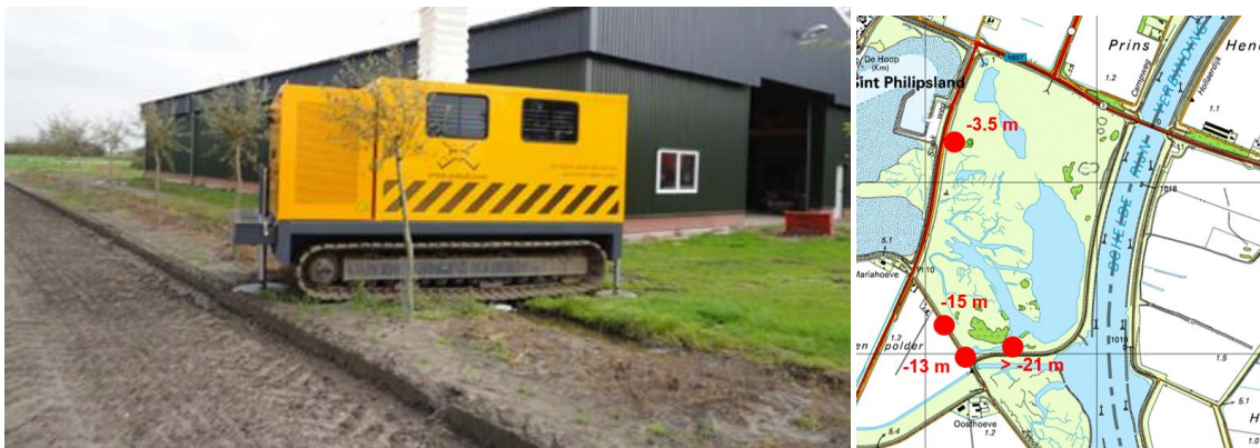
Figure 18. ECPT-vehicle to carry out Electrical Cone Penetration Tests (left). Locations of the ECPT-measurements with depth of the fresh-salt interface (right).
