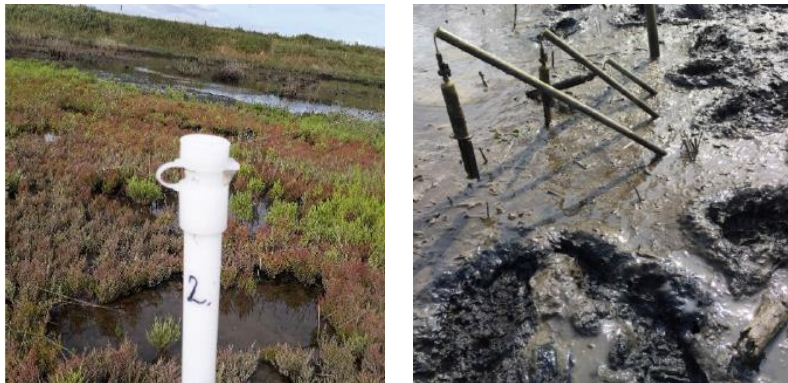
Figure 54. Sampling location 2 and monitoring well (a); Macro-Rhizon soil moisture samplers monitoring location 12 (b).
