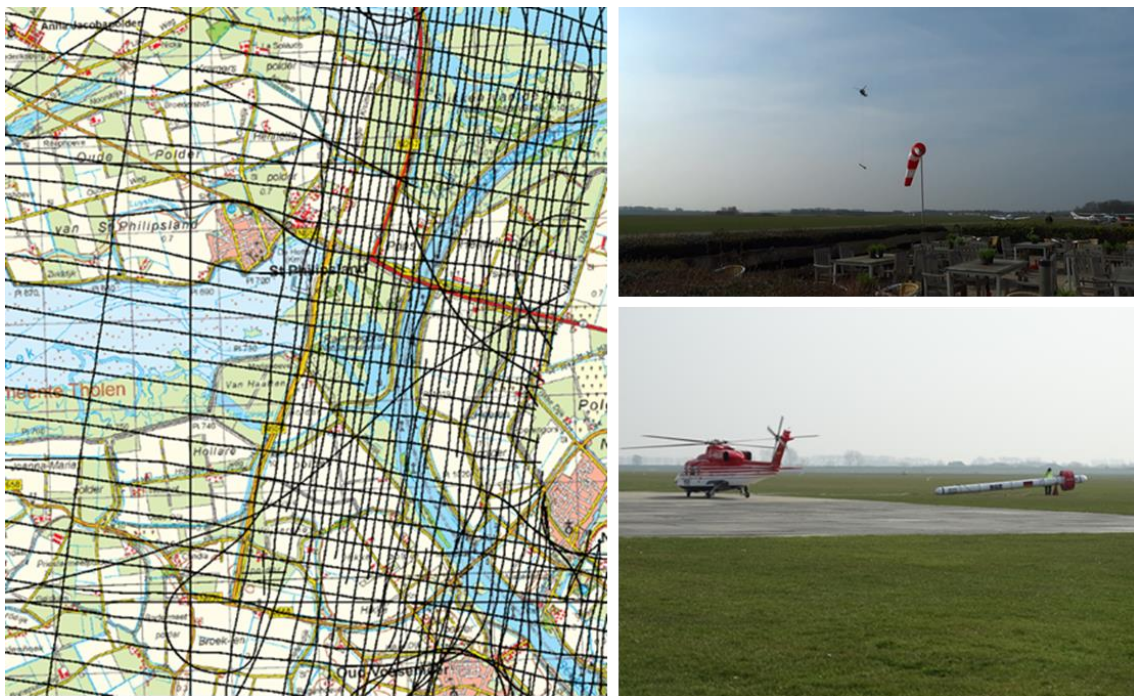
Figure 22. The flight lines (March 2015) with much narrow spacing above the Rammegors area (left). Helicopter with bird coming back to Airport Zeeland from survey above Rammegors. Helicopter with bird at Airport Zeeland ready to take off to map the salinity distribution at and around Rammegors.
