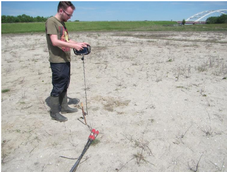
Figure 81. Use of the Eijkelkamp penetrometer.
