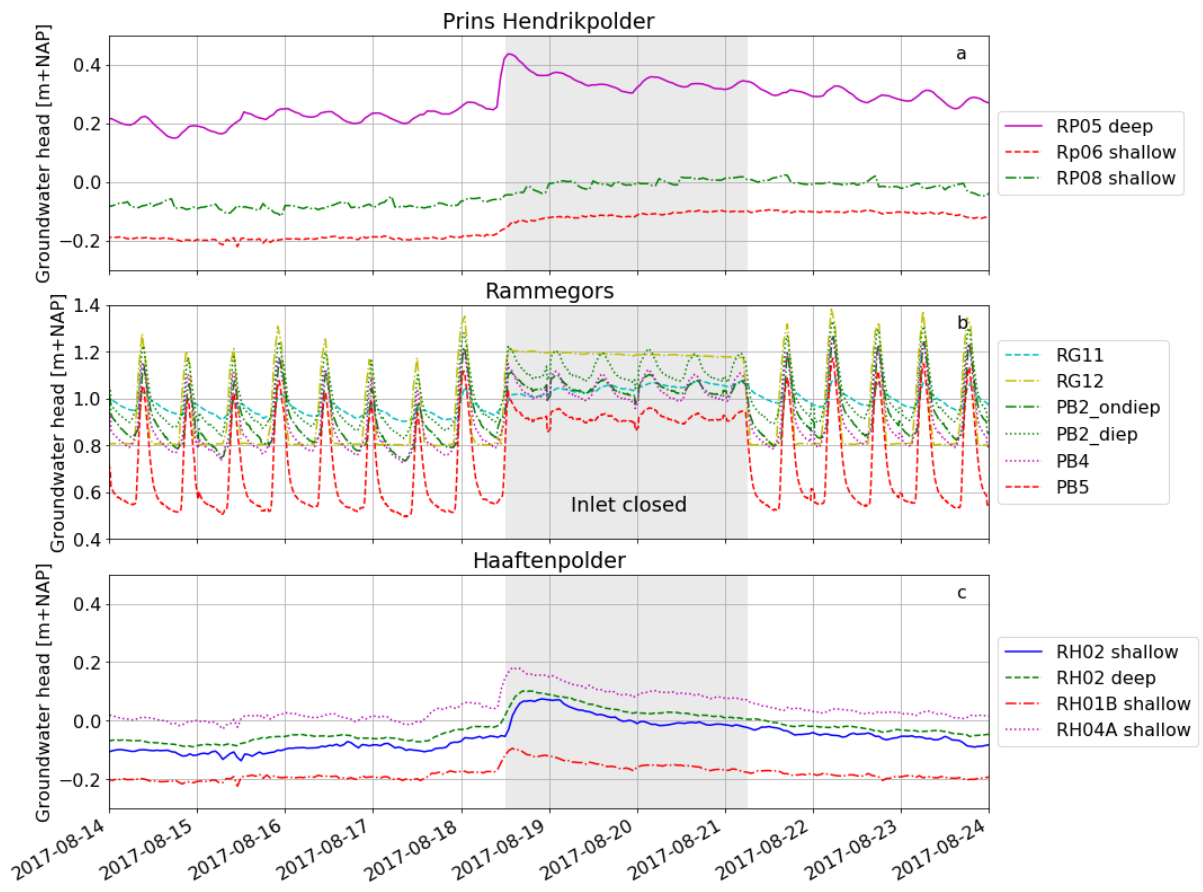
Figure 27. Groundwater heads in meter above NAP in the Prins Hendrikpolder (a), Rammegors area (b) and Haaftepolder (c) during the closure of the inlet in August 2017.
